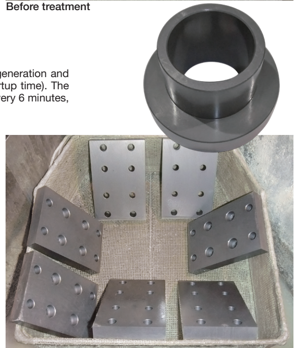
After zinc phosphate (Fericat) treatment
